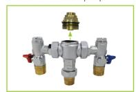
Step 7. Unscrew the brass top cap. Install the thermostatic element and spring inside the body of the valve, screw on the top cap back in place.
