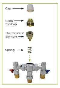
Step 8. Open the intel ball valves of the valve.
