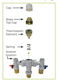
Step 3. Remove strainer cap and take out strainer, then flush your line for at least 5 minutes, then clean the strainer and reinstate in position.
