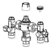
Step 6. Return the cold water knob to the open position.
