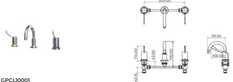
Zero Lead Stainless Steel 316 Hob Mounted 100mm Lever Basin Set w/ Curved Fixed Spout
