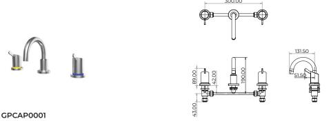
Zero Lead Stainless Steel 316 Hob Mounted 25mm Handle Basin Set w/ Curved Fixed Spout
