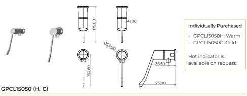
Zero Lead Stainless Steel 316 Wall Mounted 150mm Lever Cistern Tap
